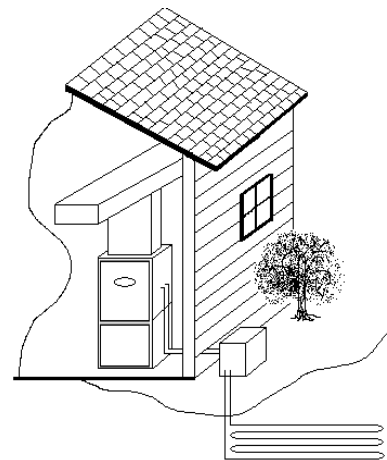
Figure 9: Split GCHP system
